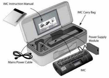
Figure 2 - Parts for the IMC
